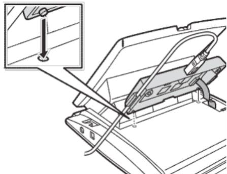
6. Attach the KX-DT301 to your unit with the screws (included with KX-DT301).
