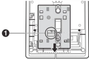
3. Attach the wall mounting adaptor as shown.
