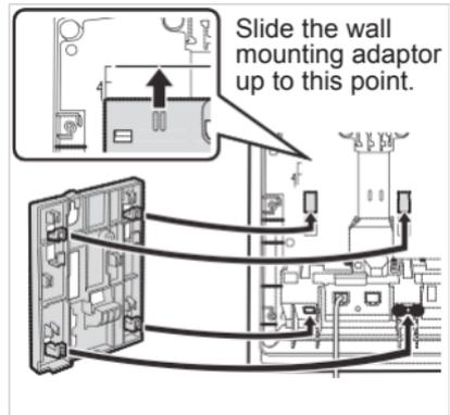
4. Drive the 2 screws (included) into the wall either 83 mm or 100 mm apart, and mount the unit on the wall.
